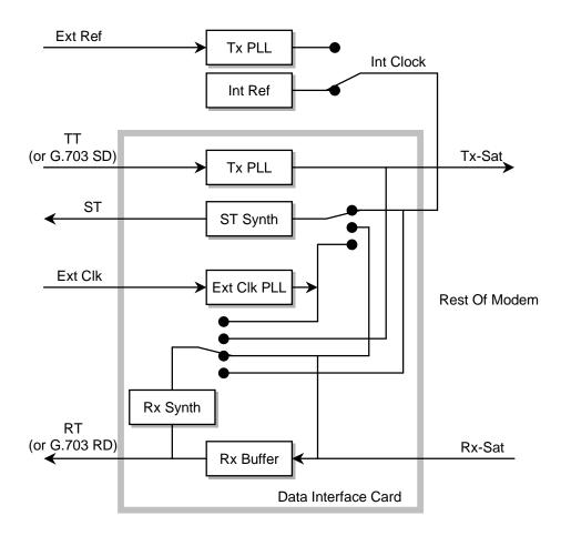
Figure 8-1. Typical Data Interface (Features Vary By Interface)
