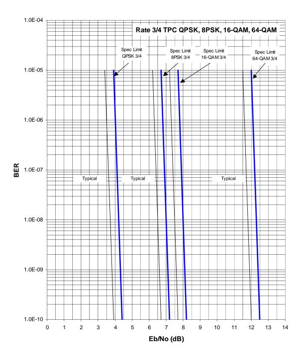
Figure 7-3. Rate 3/4 TPC QPSK, 8-PSK, 16-QAM, 64-QAM
