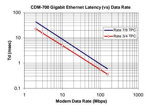
Figure 7-1. CDM-700 Gigabit Ethernet Latency with Modem in IF Loopback
