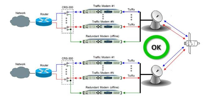
Figure 14-5. Wired-thru for Hub-to-Hub with Standard Traffic using Routers
