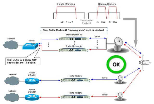
Figure 14-13. Point-to-Multipoint using Switches
