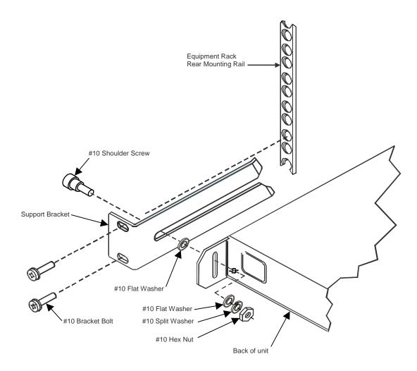
Figure 2-1. Installation of Optional Rear-Mounting Support Brackets (Kit KT/6228-2)
