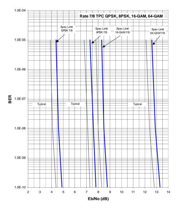
Figure 7-4. Rate 7/8 TPC QPSK, 8-PSK, 16-QAM, 64-QAM
