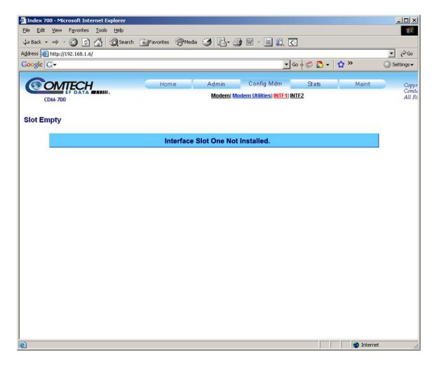
Figure 15-8. Config Mdm: INTF1 Page (Default – no module installed)
