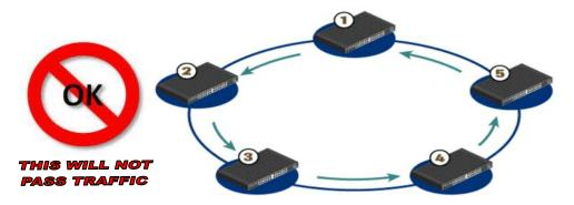
Figure 14-1. Networking Loop with Switches
