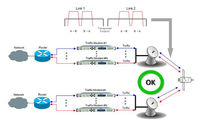
Figure 14-4. Hub-to-Hub with Standard Traffic using Routers
