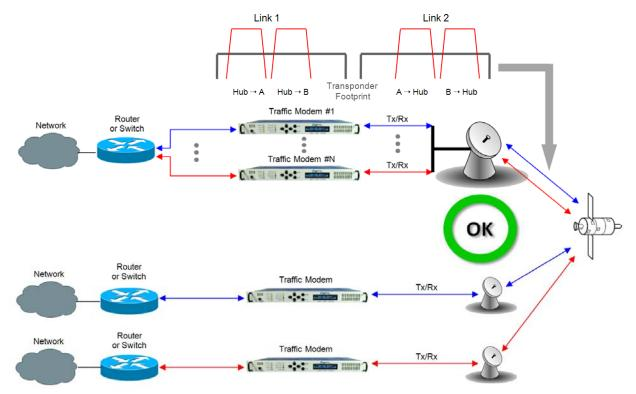
Figure 14-7. Hub-to-Remotes with Standard Traffic using Routers or Switches
