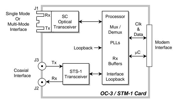
Figure C-1. Optical / Coaxial Interface Block Diagram
