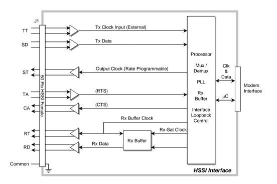
The CDI-60 HSSI Interface has a single rate programmable port. Figure 8-4 shows the interface.
