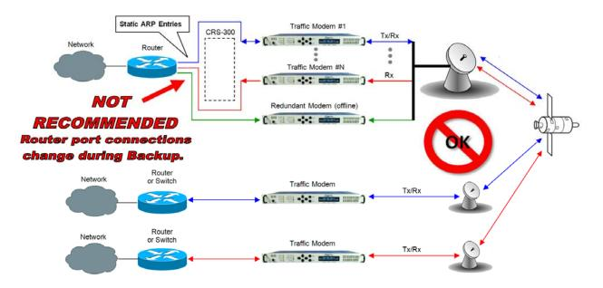
Figure 14-12. Wired-around for Point-to-Multipoint with Routers
