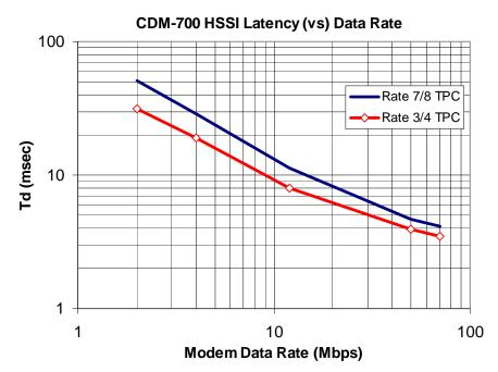
Figure 7-2. CDM-700 HSSI Latency with Modem in IF Loopback
