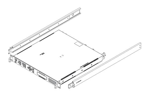
Figure 2-2. Installation of Optional Side-Railings (FP/SL0006)
