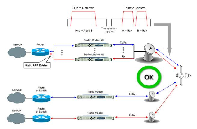
Figure 14-10. Point-to-Multipoint using Routers
