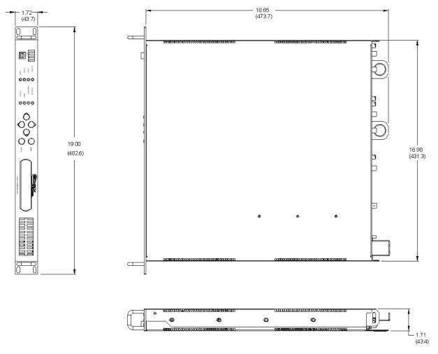
Figure 4-3. CDM-700 Dimensional Envelope (70/140 MHz)
