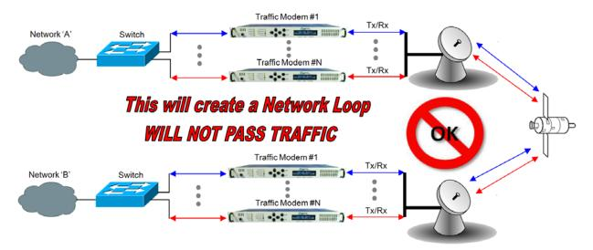
Figure 14-2. Networking Loop Example
