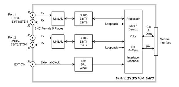
Figure B-1. Block Diagram of Dual E3/T3/STS-1 Data Interface Module
