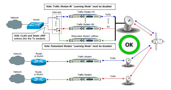
Figure 14-14. Wired-thru, Hub-to-Remotes, Split-path Traffic using Switches (Point-to-Multipoint)
