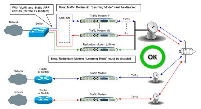
Figure 14-15. Wired-around, Hub-to-Remotes, Split-path Traffic using Switches (Point-to-Multipoint)
