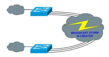
Figure 14-3. Networking Loop Example (Simplified)
