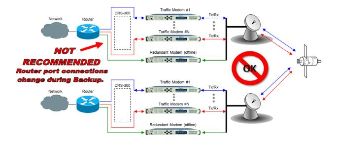
Figure 14-6. Wired-around for Hub-to-Hub with Standard Traffic using Routers
