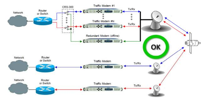
Figure 14-8. Wired-thru for Hub-to-Remotes with Standard Traffic using Routers or Switches
