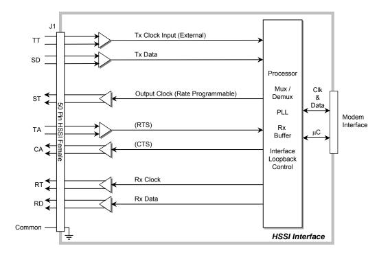
Figure D-1. HSSI Interface Block Diagram
