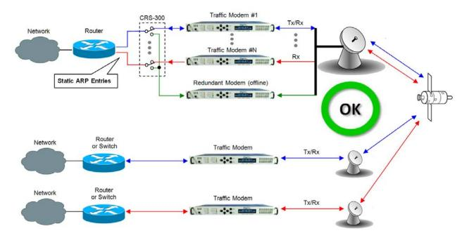
Figure 14-11. Wired-thru for Point-to-Multipoint with Routers
